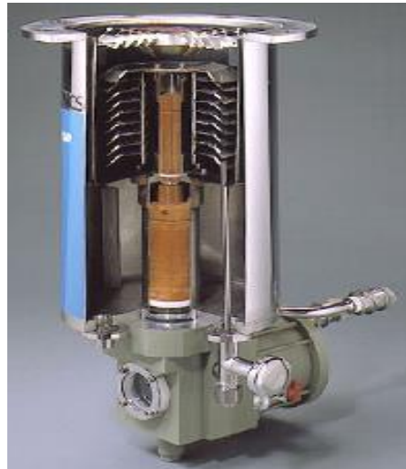
Helix CTI-10; pumping speed (N 2 ) 3000 l/sec
