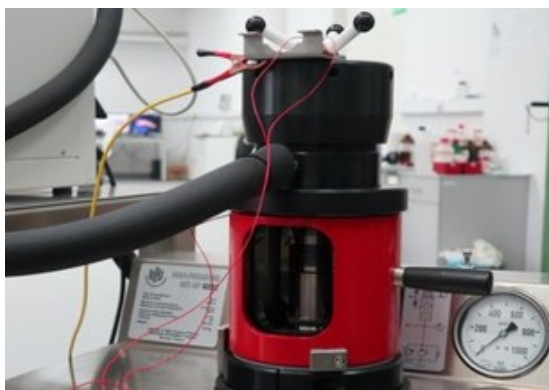
Figure 5. High-Pressure (up to P = 2.4\text{ GPa} , -20\text{ }^{\circ}\text{C} < T < 150\text{ }^{\circ}\text{C} , V = 10\text{ mL} ) set up for in-situ Broadband Dielectric Spectroscopy (BDS) tests. Special liquid as a medium transmitting pressure. The facility available in IHPP PAS 'Unipress', X-Press-Matter Lab, Warsaw, Poland ( https://young4softmatter.pl/ )
