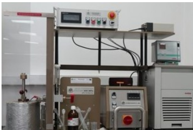
Figure 4. High-Pressure (up to 0.9 GPa, -30\text{ }^{\circ}\text{C} < T < 150\text{ }^{\circ}\text{C} , V = 20\text{ mL} ) setup for in-situ Broadband Dielectric Spectroscopy (BDS), DTA and density tests. A special liquid serving as a pressure-transmitting medium is required. The high-pressure chamber is the silver element on the left. In the center, a high-pressure pump and the control system are visible. On the right, a large-volume thermostat with external circulation is visible. The facility is available in IHPP PAS 'Unipress', X-Press-Matter Lab, Warsaw, Poland ( https://young4softmatter.pl/ )
