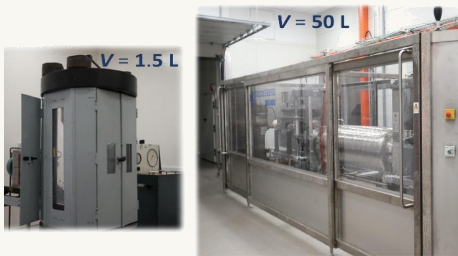
Figure 3: Processor for high-pressure preservation/processing (HPP) with pressure chambers of different volumes, as indicated in the figure. Facilities in X-PressMatter Lab IHPP PAS [38]. They are lab-scale (left) and pilot-scale (right) facilities, with the volumes of the pressure chambers shown in the plot. The operation up to P = 600\text{MPa} .
