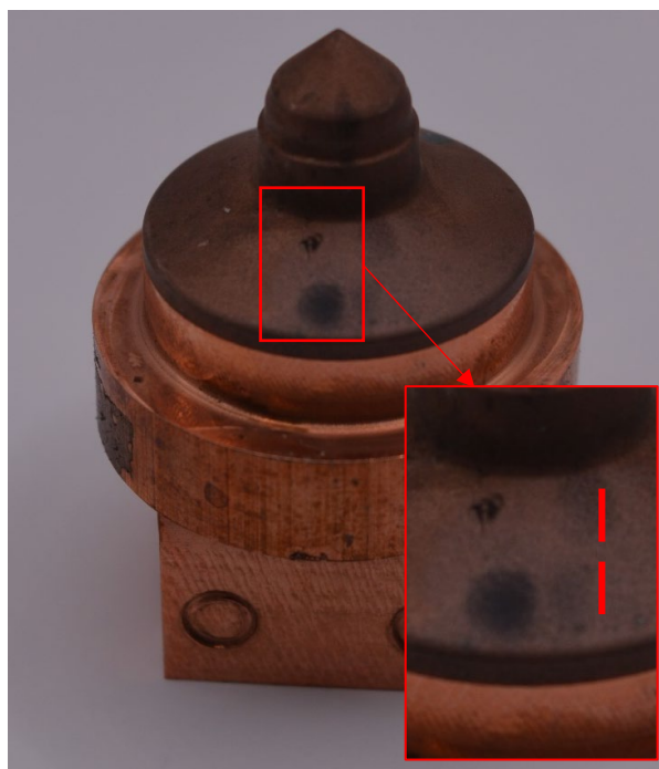
Figure 8. View of the G2 electrode with the marked measuring section, lc .
