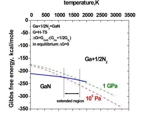
The equilibrium  $p_{N2} - T$  conditions for GaN were determined by direct synthesis and decomposition experiments performed by both: gas-pressure technique and highpressure anvil technique.
