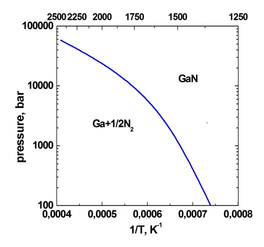
The experimental nitrogen solubility data result from annealing of Ga in N<sub>2</sub> atmosphere at three phase Ga-N<sub>2</sub>-GaN equilibrium conditions.
