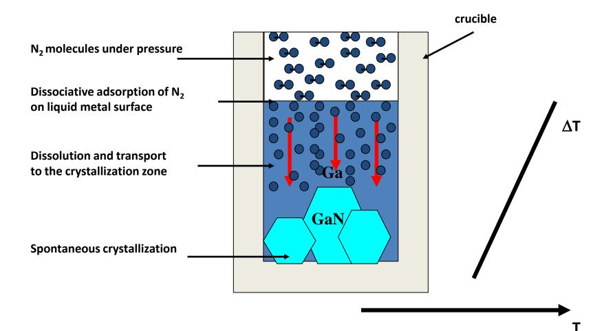
The GaN crystals are grown spontaneously from the wall of the crucible, from the GaN polycrystalline layer (film) created on the surface of the liquid metal.
